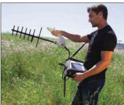
▲ Fig. 6 Direction finding in the field with a handheld spectrum analyzer and unidirectional antenna.
