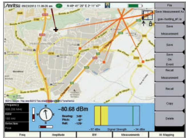
▲ Fig. 7 Triangulation locates the source of interference on the instrument's map.
