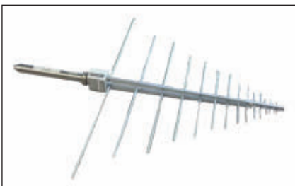
▲ Fig. 3 A Log Periodic antenna can capture a variety of interferers across a wide frequency spectrum.
